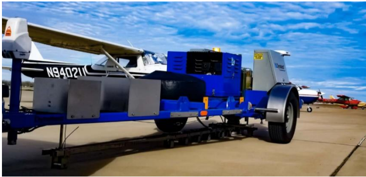
FIGURE 3-3: HEAVY WEIGHT DEFLECTOMETER
