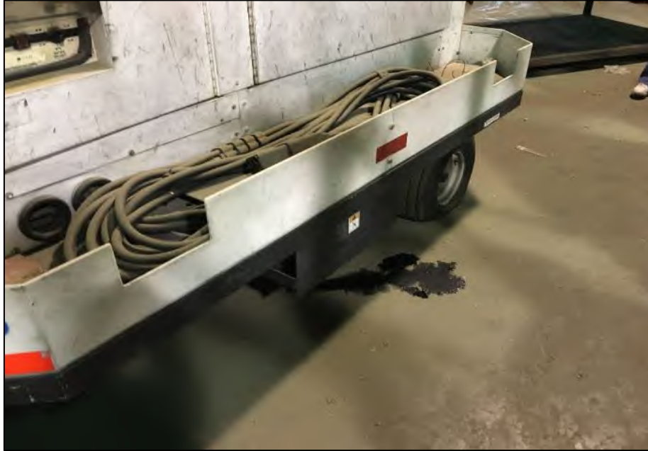
Inside of 61W-32, building #4. Leaking aircraft cart.
