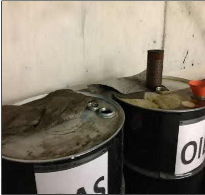
Oil and gas drums inside the Guardian Center southern hangar with no bungs, absorbent pads and used oil filters.
