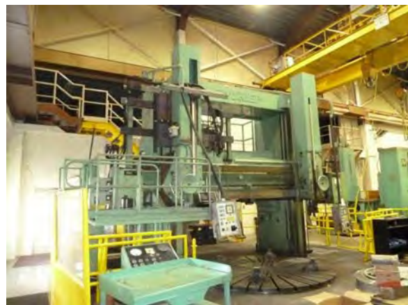
Photo of the 120-inch Froriep Vertical Turning Lathe (above) and the 5-inch G&L Horizontal Boring Mill (below) in the La Verne Machine shop.
